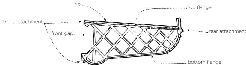
**STEP 7:** Attach Can Tracks to the frame. Depending on which configuration you purchased, you may have one, two, or all three sizes of Can Tracks. If you have different sizes of Can Tracks, remember to put the large Can Tracks on the bottom, medium Can Tracks in the middle, and small Can Tracks on the top.
