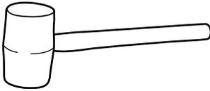
**Note:** use a hard rubber or plastic mallet to pound metal pieces together (a hammer may leave dents and chips in the paint).
