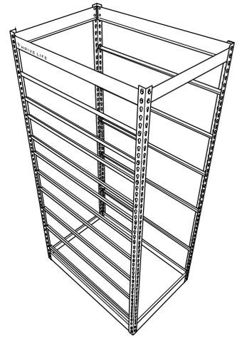
**STEP 6:** Attach the remaining wide beam (with logo) to the front side of the frame in the top two notches on the angle posts.
