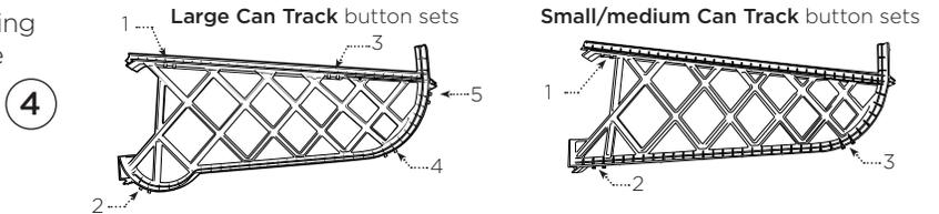
5. Connect adjacent Can Tracks by alternating straps between the top and bottom sets of buttons, as shown below.
