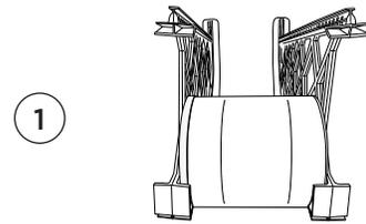
2. Adjust the width of the Can Tracks along the crossbars so that the can rests about 1/8" away from the center rib of the Can Track on each side.
