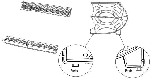
**2.** Press the first track downward so the posts fit firmly into hole #1 on the brackets.
